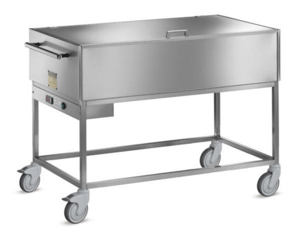
Bain-marie heated trolley for distribution of meals (GN not included). Welded frame made in stainless steel 18/10 AISI 304. Double-wall basin. Bain-marie electric water-bath heating 2000 W - 230 V. Temperature controlled by a mechanical thermostat 30° - 90° C°. Spiral cable with "Schuko" plug. 4 grey not marking, rubber swivelling wheels, 2 with brake Ø 125 mm. Trolley capacity 4GN 1/1 h 200 (60 - 80 meals) mm 1500x640x900 h - 026.AD/M
