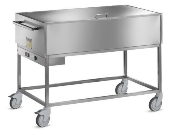
Bain-marie heated trolley for distribution of meals (GN not included). Welded frame made in stainless steel 18/10 AISI 304. Double-wall basin. Bain-marie electric water-bath heating 2000 W - 230 V. Temperature controlled by a mechanical thermostat 30° - 90° C°. Spiral cable with "Schuko" plug. 4 grey not marking, rubber swivelling wheels, 2 with brake Ø 125 mm. Trolley capacity 3GN 1/1 h 200 (50-60 meals) mm 1200x640x900 h - 026.AC/M
