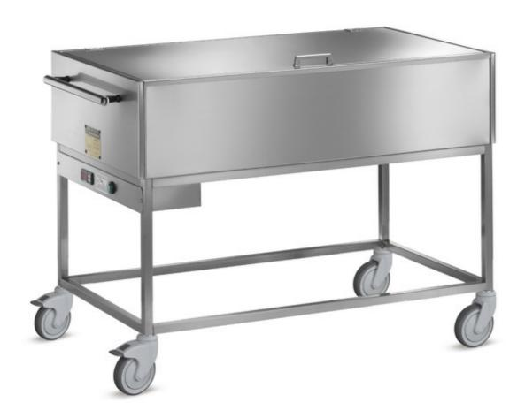
Bain-marie heated trolley for distribution of meals (GN not included). Welded frame made in stainless steel 18/10 AISI 304. Double-wall basin. Bain-marie electric water-bath heating 2000 W - 230 V. Temperature controlled by a digital thermostat 30° - 90° C°. Spiral cable with "Schuko" plug. 4 grey not marking, rubber swivelling wheels, 2 with brake Ø 125 mm. Trolley capacity 1 GN 1/1 h 200 (15-20 meals) mm 710x450x900 h - 026.AA
