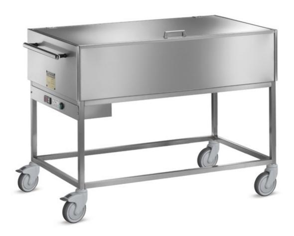
Bain-marie heated trolley with lid and without undershelf, carrying frame made in stainless steel 18/10 AISI 304. Stainless steel basin with grid for containers support. Electric water-bath heating, 2000W - 230 V. Temperature controlled by a digital thermostat 30° - 90° C°. Spiral cable with "Schuko" plug. 4 grey not marking, rubber swivelling wheels, 2 with brake Ø 125 mm. Bain-marie heated trolley 2000W mm 1200x640x900 h - 013.A
