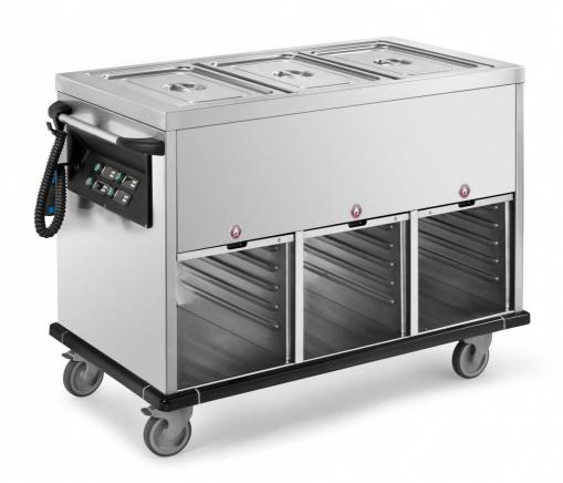
Heated bain-marie trolley unique basin, structure completely made in stainless steel 18/10 AISI 304, dry/bainmarie heating, temperature controlled by digital thermostat 30° - 90° C°. Printed unique basin with rounded corners, for 2 GNI/1 h 200, anti-drop board, insulated double wall, spiral electrical wire with CE plug and hooker for the plug, ergonomic push handle. Under compartments with hiding tilting doors, with 5 printed slideways, pitch 55mm, capacity 2 GNI/1 h 100 mm + 1
