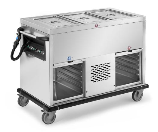
HEATED TROLLEY WITH UNIQUE BAINMARIE BASIN - HEATED AND/OR REFRIGERATED UNDERCOMPARTMENTS, structure completely made in stainless steel 18/10 AISI 304, dry/bainmarie heating, temperature controlled by a digital thermostat 30° - 90° C° heated section and +4°/+10° C° refrig. section - 230 V 50/60 Hz. Unique deep-drawn basin with rounded corners for GN1/1 H 200, anti-drop board, insulated double wall. Spiral electrical wire with CE plug and hooker for the plug,
