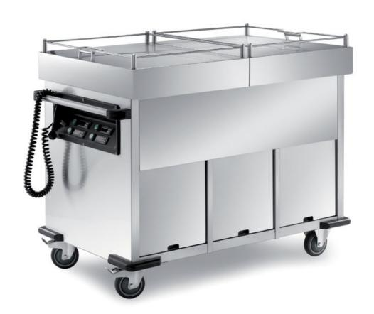
Heated bain-marie trolley unique basin with sliding lids (GN not included), structure completely made in stainless steel 18/10 AISI 304 dry/bainmarie heating, Temperature controlled by digital thermostat 30°-90° 230V 50/60Hz. Insulated lids are opening up to 180°. Printed unique basin with rounded corners, for 3 GN1/1 H 200mm, anti-drop board, insulated double wall, Spiral electrical wire with CE plug and hooker for the plug, ergonomic push handle. Under compartments with
