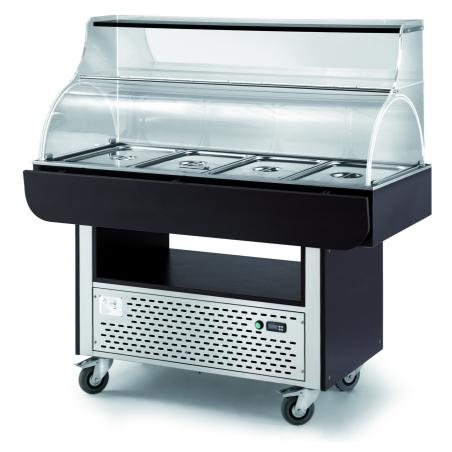
Wall refrigerated display cabinet, wengé colour (GN not included) stainless steel structure with wengé panels. Pressed bowl with antidrop border. Plexiglas superstructure with semicylindric dome. Hermetic refrigerating system HP 1/8 500W 230V 50/60Hz single-phase. Digital temperature control 0°-15°C. 4 wheels, Ø 125 mm, 2 of which with brakes. Capacity 3GN 1/1 h 150. Capacity 4 GN 1/1 h 200 mm - 500 W; dim. mm 1500x640x1400 h - 715.P
