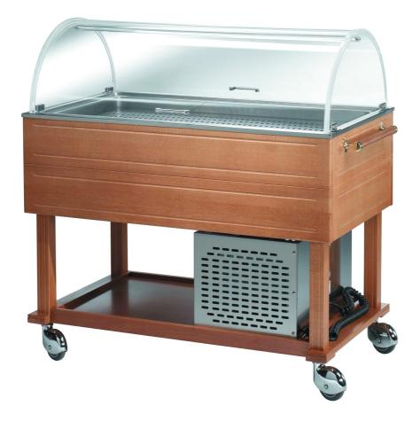
Refrigerated trolley (GN not included), Carrying frame and shelves made in solid wood. Pressed no-drops basin made in stainless steel 18/10 AISI 304. Dome made in transparent plexiglass. Hermetic circuit refrigerating system, consisting of HP 1/8 500 W - 230 V, single-phase compressor unit. The temperature is controlled by a digital thermostat approx. -5°+10° C. 4 swivelling wheels covered with casing Ø 100 mm. Refrigerated trolley, semi-cylindrical dome, capacity 3 GN 1/2 h 200
