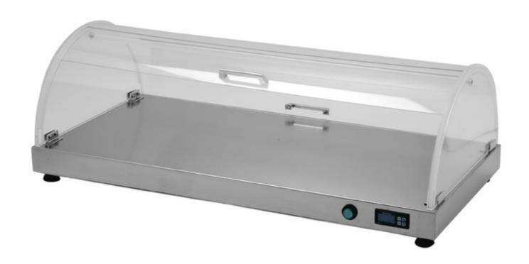
Hot shelves with dome, made in stainless steel 18/10 AISI 304, heating by electrical contact resistance 230 V, warning light, digital thermostat 30°-90° C, squared dome 500 W, dim. mm 1000x500x250 h - PCCQ/3
