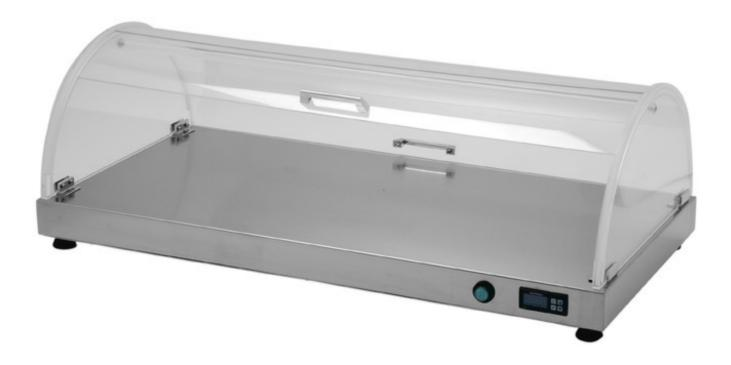
Hot shelves with dome, made in stainless steel 18/10 AISI 304, heating by electrical contact resistance 230 V, warning light, digital thermostat 30°- 90° C, squared dome 450 W, dim. mm 900x500x250 h - PCCQ/2
