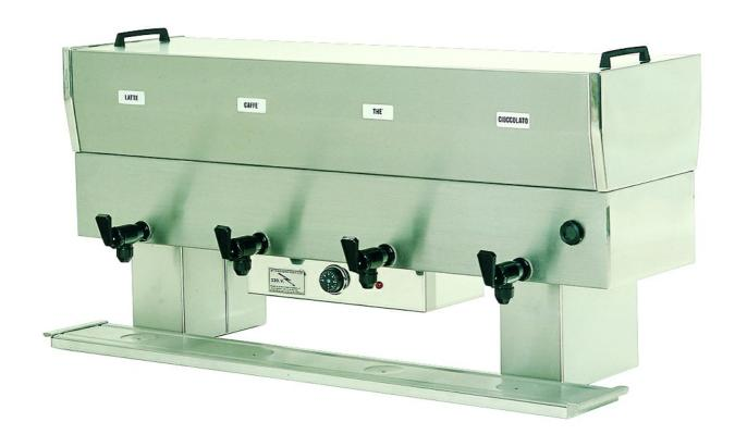
Heated breakfast distributor, made in 18/10 stainless steel. Pots made in 18/10 stainless steel with lids, capacity 10 lt. Plastic taps can be easily desmounted for daily cleaning; basin to collect drops. Electric waterbath heating 2000 W - 230 V. Temperature controlled by a digital thermostat 30°- 90° C and warning light. Little feet made in stainless steel 18/10. Distributor 2000 W, capacity 4 containers 10 lt, dim. mm 1180x420x600 h - 744.A4
