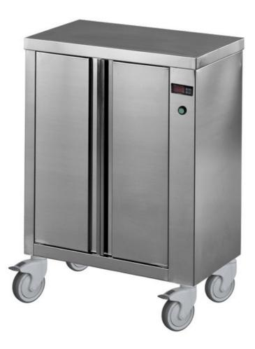
Dish-warmer trolley, frame made in stainless steel 18/10 AISI 304, isolated. Intermediate shelf and heat-retaining swing door.Ventilated heating controlled by a digital thermostat 30°- 90° C. 1000 W - 230 V 50/60 Hz. 4 grey not marking rubber swivelling wheels Ø 125 mm, 2 with brake. Dish-warmer trolley, 2 swing doors, capacity 150-200 dishes Ø 320 mm. Dim. mm 820x390x910 h - 791.A
