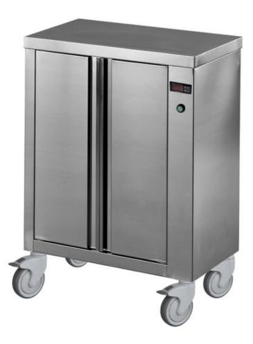
Dish-warmer trolley, frame made in stainless steel 18/10 AISI 304, isolated. Intermediate shelf and heat-retaining swing door.Ventilated heating controlled by a digital thermostat 30° - 90° C. 1000 W - 230 V 50/60 Hz. 4 grey not marking rubber swivelling wheels Ø 125 mm, 2 with brake. Dish-warmer trolley, 1 swing door, capacity 100 dishes Ø 320 mm. Dim. mm 520x390x910 h - 790.A
