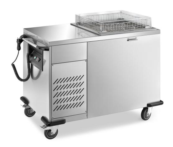
Ventilated refrigerable basket elevator with 1 column -2/+8°C. Entirely made in 18/10 stainless steel with 2 fixed wheels and 2 swivelling with brake diam 125 mm and corner bumper. Lids included. Digital thermostatic regulation +30° - +90°C, 607 W - 230 V 50/60 Hz. Capacity basket 6, dim mm 500x500x115 h or capacity basket 9, dim mm 500x500x75 h - CSR5/5
