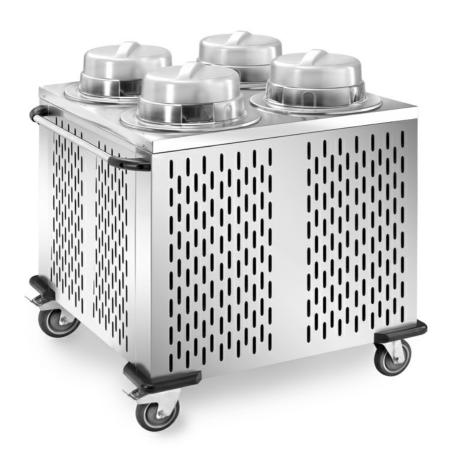
Refrigerable dishes distributor with 4 adjustable columns. Entirely made in 18/10 stainless steel with 2 fixed wheels and 2 swivelling with brake diam. 125 mm and corner bumper. Lids included. Capacity 200-240 dishes, diam 28/32 Dim. mm 1030x990x1060 h - CSG/4F
