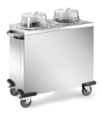
Dishes distributor with 2 fixed columns. Entirely made in 18/10 stainless steel with 2 fixed wheels and 2 swivelling with brake diam. 125 mm and corner bumper. Lids included. Capacity 100-120 dishes, diam 16/21. Dim. mm 930x480x1060 h - CSL/2N
