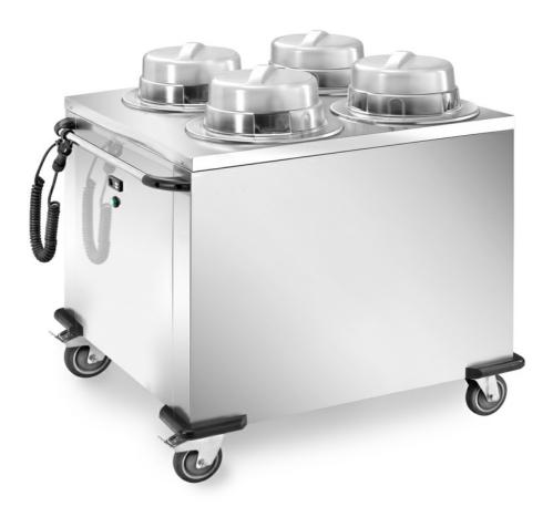
Heated dishes distributor with 4 adjustable columns. Entirely made in 18/10 stainless steel with 2 fixed wheels and 2 swivelling with brake diam. 125 mm and corner bumper. Lids included. Digital thermostatic regulation +30° - +90°C, 2000 W - 230 V 50/60 Hz. Capacity 200-240 dishes, diam 18/28 Dim. mm 1030x900x1060 h - CSP/4C
