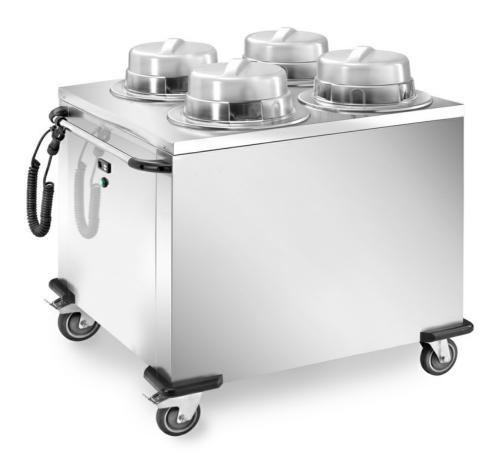
Heated dishes distributor with 4 fixed columns. Entirely made in 18/10 stainless steel with 2 fixed wheels and 2 swivelling with brake diam. 125 mm and corner bumper. Lids included. Digital thermostatic regulation +30° - +90°C, 2000 W - 230 V 50/60 Hz. Capacity 200-240 dishes, diam 16/21 Dim. mm 1030x900x1060 h - CSL/4C
