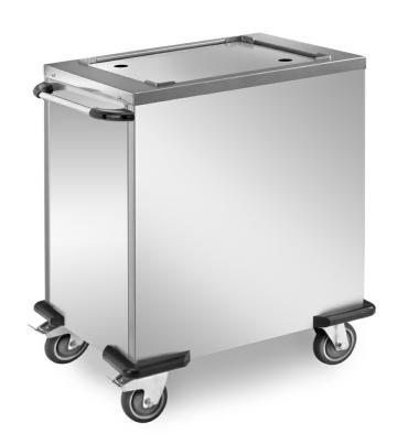
Elevator trolley with universal platform. Structure in stainless steel 18/10 AISI 304. With handle and black PVC bumpers. On 4 wheels Ø 125, 2 fixed and 2 with brake. Elevation top dimension mm 580x340 for trays 570x325. - CPV57/32
