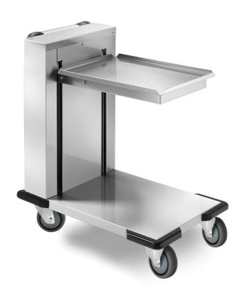
Elevator for trays and baskets. Entirely made in 18/10 stainless steel, Capacity 120-150 trays and 6 baskets h. 115 or 9 baskets h. 75; 4 wheels diam 125 mm, 2 fixed and 2 swivelling with brake. Dim trays 1 GN2/1 - 2 GN1/1 mm 500x500. Dim mm 850x560x900 h - PV52/65
