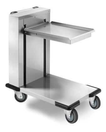
Elevator for trays and baskets. Entirely made in 18/10 stainless steel, Capacity 120-150 trays and 6 baskets h. 115 or 9 baskets h. 75; 4 wheels diam 125 mm, 2 fixed and 2 swivelling with brake. Dim Baskets mm 500x500. Dim mm 850x560x900 h - PV52/52
