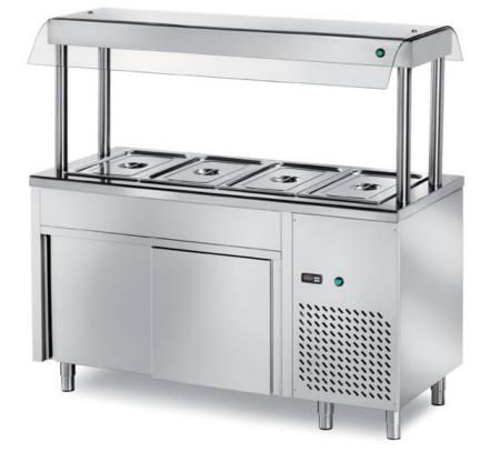
Refrigerated central island, with a h 200 bowl - with neutral sliding doors cabinet + motor compartment with 1 control. Upper shelf equipped with curved glass and with internal lighting - GN containers not included, mm 1500x700x1500 h - SIN/15
