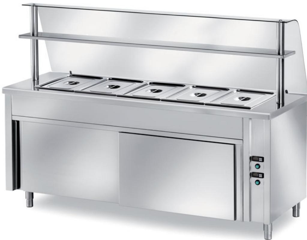
Self service heated table, heated and ventilated cabinet, 3000 Watt, half-rounded basin H200, capacity 4 basins GN 1/1 h 150 (GN not included) mm 1500x800x1400 h + curved toughened glass - SFC8/15
