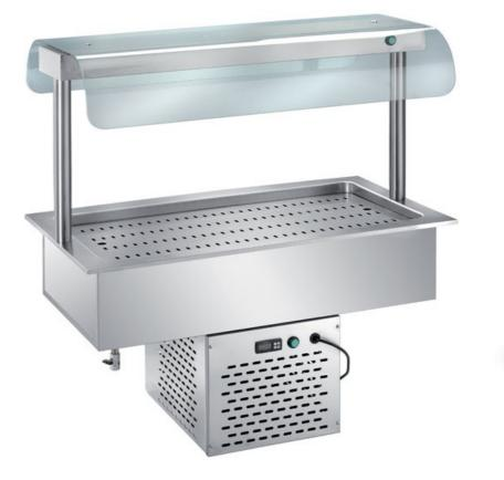
Static refrigerated drop-in basin mm.200h, temperature -2�/+15�C, with upper toughened glass with lights, dim. mm.1480x640x820h -212W - cap. 4GN1/1 h 200 - 140.TN
