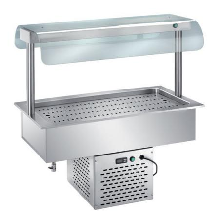
Static refrigerated drop-in basin mm.200h, temperature -2 \( \psi / + 15 \) C, with upper toughened glass with lights, dim. mm.900x640x820h - 170W - cap. 2GN1/1 h 200 - 100.TN
