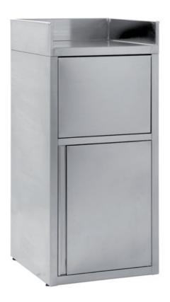
Self service feedbox for trays unloading. Upper self with raised top h. 150 mm. on 3 sides - under compartment with swing door for dustbin CRC/2 - Swinging door for trays unloading mm 600x600x1300 h - TRC/2
