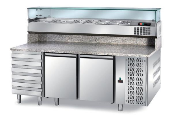
Refrigerated table 3 swing doors, worktop made in granite, backsplash, refrigerated unit for containers with glass (containers not included), incorporated motor, mm 2140x800x1400h - TPF3/21
