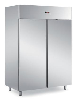
Refrigerated cabinet TN in stainless steel AISI 304 18/10, Lt. 1400, insulation thickness 75 mm with 3 plastic grids mm. 530x650, automatic defrosting and condensation evaporation, digital control. Temp. -2/+10°C dim. mm 1420x800x2050 h - GP500
