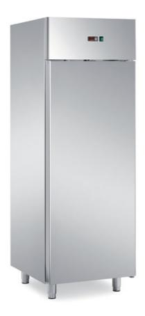
Refrigerated cabinet TN in stainless steel AISI 304 18/10, Lt. 700, insulation thickness 75 mm with 3 plastic grids mm. 530x650, automatic defrosting and condensation evaporation, digital control. Lighting and keys included, Temp. -2/+10°C dim. mm 710X800X2050 h - GS250
