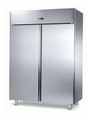
Refrigerated cabinet TN with 2 doors, Lt. 1400 temp. -2°/+8°C, lighting and keys included, dim. mm 1480x830x2010 h insulation thickness 60 mm with 3 plastic grids mm. 530x650, automatic defrosting and condensation evaporation, digital control. - GT500
