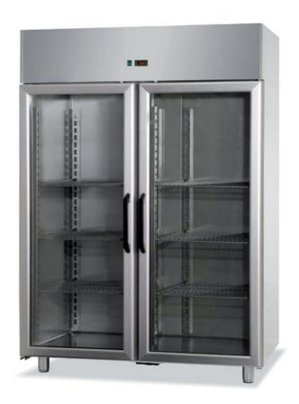
Refrigerated cabinet BT in stainless steel AISI 304 18/10, Lt. 1400, insulation thickness 75 mm with 3 plastic grids mm. 530x650, automatic defrosting and condensation evaporation, digital control. Glass doors. Temp. -10/-20°C dim. mm 1420x800x2050 h - GVF500
