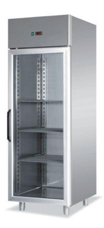
Refrigerated cabinet BT in stainless steel AISI 304 18/10, Lt. 700, insulation thickness 75 mm with 3 plastic grids mm. 530x650, automatic defrosting and condensation evaporation, digital control. Glass door. Temp. -10/-20°C dim. mm 710x800x2050 h - GVF250
