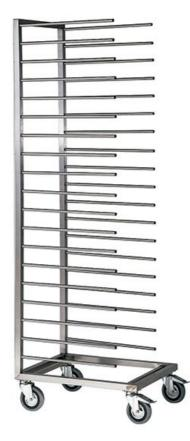
Trolley for baking tin. Welded frame made in stainless steel 18/10 AISI 304, square tube 30x30 mm. Rounded handle. 4 swivelling wheels Ø 125 mm. Capacity 16 baking tins 600x400 mm, distance between guides 95 mm; dim. mm 650x500x1760 h - 640.AS
