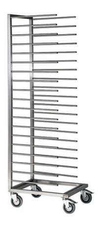
Trolley for baking tin. Welded frame made in stainless steel 18/10 AISI 304, square tube 30x30 mm. Rounded handle. 4 swivelling wheels Ø 125 mm. Capacity 20 baking tins 600x400 mm, distance between guides 80 mm: dim. mm 650x500x1860 h - 640.A
