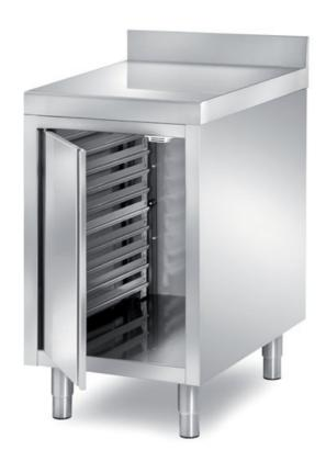
Cabinet table with I swing door with pans rack - for pans 400x600 mm and backsplash - top with rounded front edge h 60 mm dim. mm 500x700x850 h - BPF1/5A
