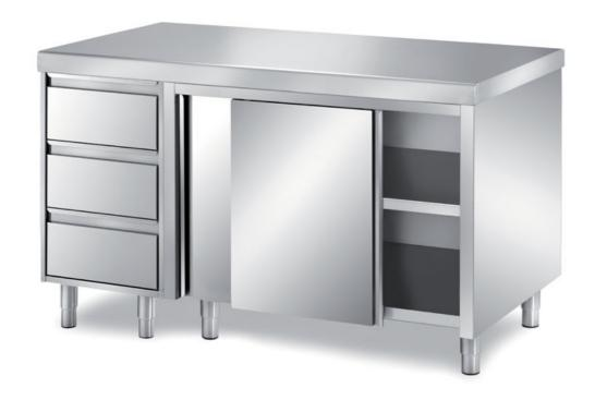
Cabinet table with sliding doors, top with rounded front edge mm 60 h adjustable middle shelf - with 1 unit with 3 drawers GN2/1 H=150mm - dim. mm 1600x900x850 h - PCC2/16
