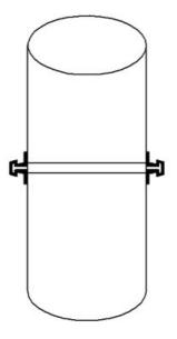
Flange for joint round ducts "tiposistem" diam. 35 STAINLESS STEEL -FLT35INOX
