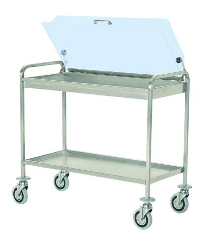
Trolley with dome, frame in square tube 20x20 mm and stainless steel shelves h 6 mm. Transparent plexiglass dome built on brake arms. 4 swivelling grey rubber castors diam. 125 mm. Trolley with 3 shelves - dim. 100x480x1100h mm - 328.A
