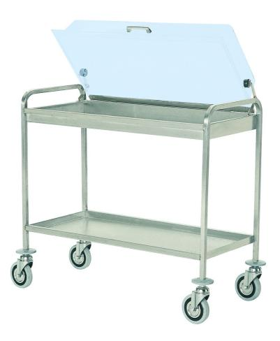
Trolley with dome, frame in square tube 20x20 mm and stainless steel shelves h 6 mm. Transparent plexiglass dome built on brake arms. 4 swivelling grey rubber castors diam. 125 mm. Trolley with 2 shelves dim. 100x480x1100h mm - 228.A
