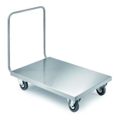
Trolley with low shelf. Carrying frame in stainles steel 18/10, with push handle, 4 castors of which 2 fixed and 2 swivelling diam 125 mm, 2 black PVC bumpers mm 600x1200x900h - 066.B
