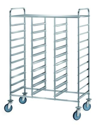
Trolley for trays with upper shelf and railing. Frame made in stainless steel 18/10 AISI 304, square tube 20x20 mm. Upper shelf and railing. 4 swivelling wheels Ø 125 mm, rubber bumpers. Capacity 30 gastronorm trays, dim. mm 1150x600x1540 h - 636.AS
