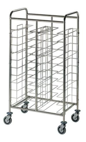
Trolley for trays, universal guides. Frame made in stainless steel 18/10 AISI 304, round tube Ø 25 mm. Guides made in chromium-plate round tube, distance between guides 11 cm. 4 swivelling wheels, rubber bumpers. Capacity 33 trays, dim. mm 1350x600x1500 - 612.U/CR
