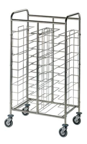
Trolley for trays, universal guides. Frame made in stainless steel 18/10 AISI 304, round tube Ø 25 mm. Guides made in chromium-plate round tube, distance between guides 11 cm. 4 swivelling wheels, rubber bumpers. Capacity 11 trays, dim. mm 450x600x1500 - 610.U/CR
