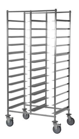
Trolley for trays. Frame made in stainless steel 18/10 AISI 304, square tube 20x20 mm. Guides shaped as "L" depth 50 mm, distance between guides 120 mm. 4 rubber swivelling wheels Ø 125 mm, 4 grey rubber bumpers. Capacity 24 euronorm trays 530x370x115 mm; dim. mm 860x600x1800 - 631.A
