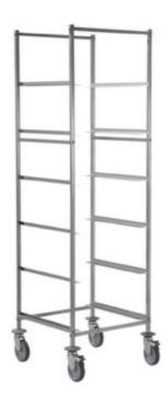
Trolley for dishwasher racks. Frame made in stainless steel 18/10 AISI 304, square tube 25x25 mm, crossbars with bolts. Guides shaped as "L" made in stainless steel, depth 50 mm and thickness 12 mm. 4 wheels Ø 125 mm, 4 grey rubber bumpers. Capacity 5 racks for dishwasher 510x510 mm, distance between guides 300 mm; dim. mm 610x570x1800 h - 633.A
