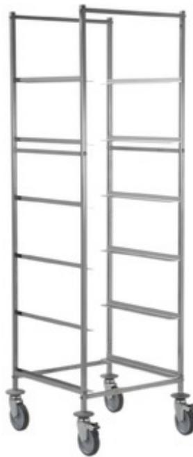
Trolley for dishwasher racks. Frame made in stainless steel 18/10 AISI 304, square tube 25x25 mm, crossbars with bolts. Guides shaped as "L" made in stainless steel, depth 50 mm and thickness 12 mm. 4 wheels Ø 125 mm, 4 grey rubber bumpers. Capacity 12 racks for dishwasher 510x510 mm, distance between guides 250 mm; dim. mm 1150x600x1800 h - 632.AS
