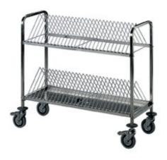
Tray-draining trolley. Carrying frame in stainless steel AISI 304 18/10, draining grids, drop-collecting basin in stainless steel with a plug. 4 swivelling castors diam. 125 mm. Stainless steel grids, cap. 60 trays dim. 1080x450x950h mm - 743
