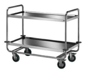
Shelves trolley made in 18/10 stailess steel, carrying frame made in 18/10 stainless steel, round tube Ø 25 mm, tray-shaped soundproof shelves made in sating 18/10 stainless steel with perfectly rounded upper and lower edges. 4 grey rubber swivelling wheels Ø 125 mm, rubber bumpers. Two-shelves trolley mm 680x680x900h - 202.AB
