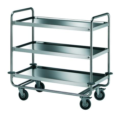
Shelves trolley made in 18/10 stailess steel, carrying frame made in 18/10 stainless steel, round tube Ø 25 mm, tray-shaped soundproof shelves made in sating 18/10 stainless steel with perfectly rounded upper and lower edges. 4 grey rubber swivelling wheels Ø 125 mm, rubber bumpers. Three-shelves trolley mm 1100x680x1020h - 313.AB
